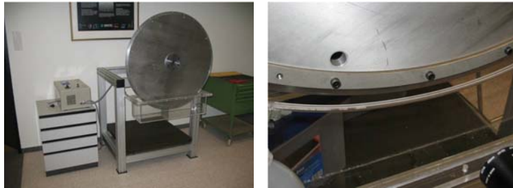
Figure 1: A rotating wheel (left) was designed with appropriate edge geometry in order to emulate the sliding wire geometry. A thermoformed plexiglass groove (right) of appropriate width was applied against the disk edge and slurry was injected into the disk-groove gap.
