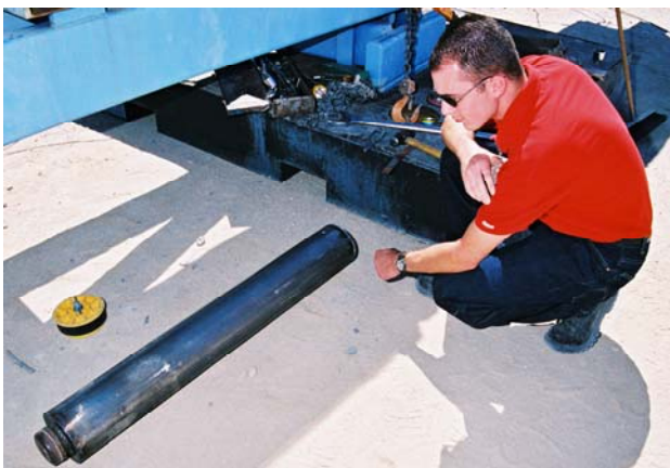
Projectile loaded with 15 liters of kerosene
