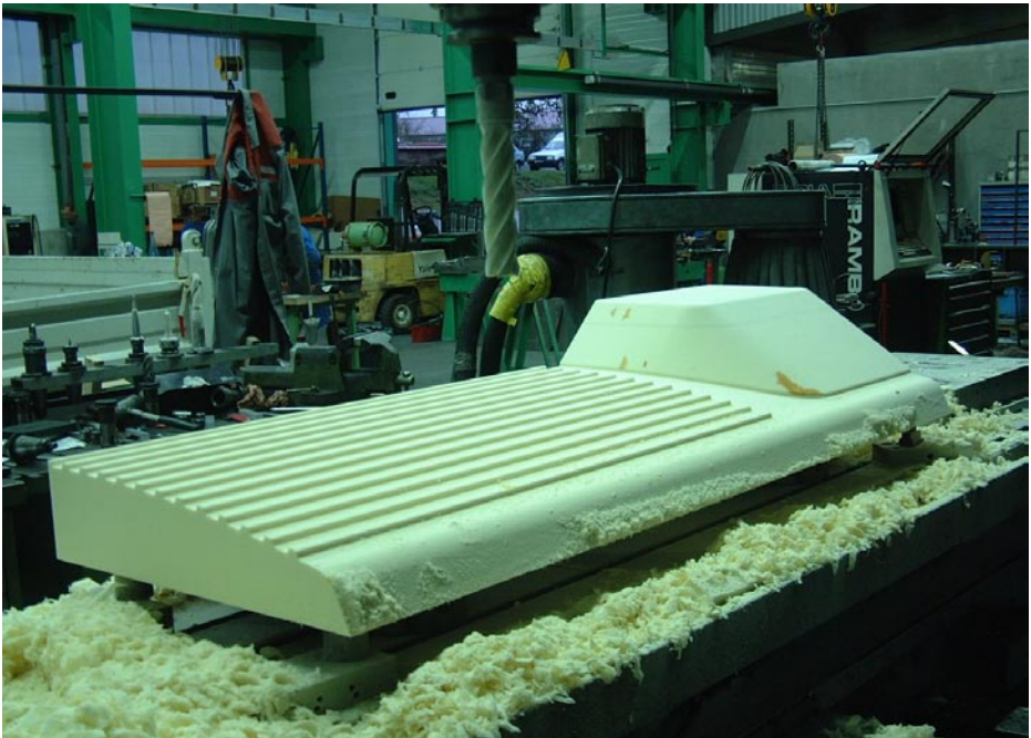
Machining of one of the models using a five-axis machine-tool
