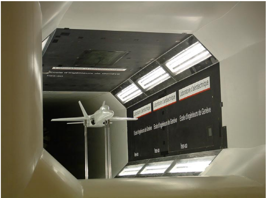
Model mounted on motor driven pylons
